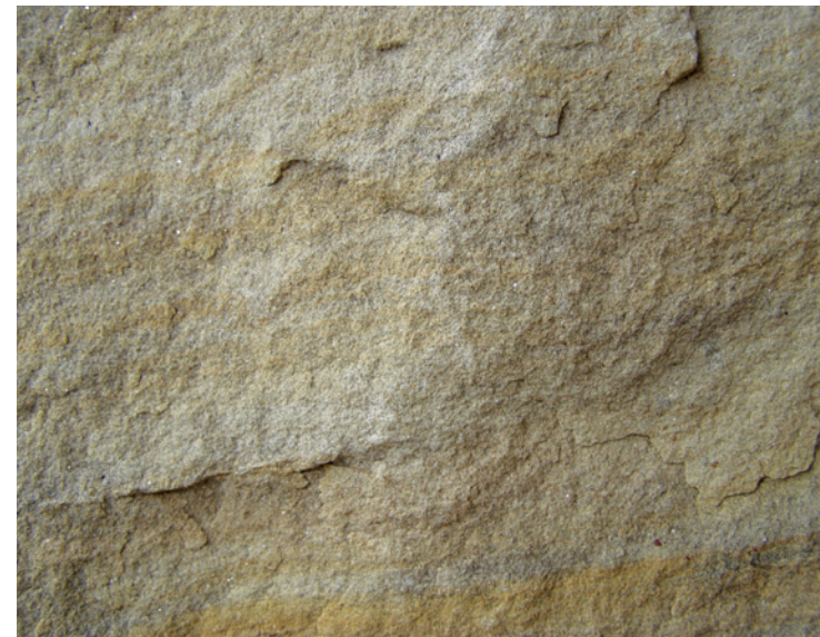
A fresh piece of sandstone with orange bands of iron oxides.
